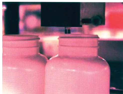
Wrapped source tags are inserted into 200cc bottles holding tablets of vitamins or dietary supplements. The bottle opening of just 1.25-inch proved to be no problem for accurate and reliable placement.
