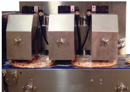
The modular construction of George Gordon and Associates Accu-wrap FG-2DDDW allows removal of all modules for expediant change-over and flexibility for future line changes.
